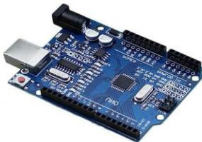
Fig 3.1:- Arduino Uno Board
