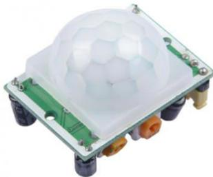
Fig 3.5: PIR sensor module
